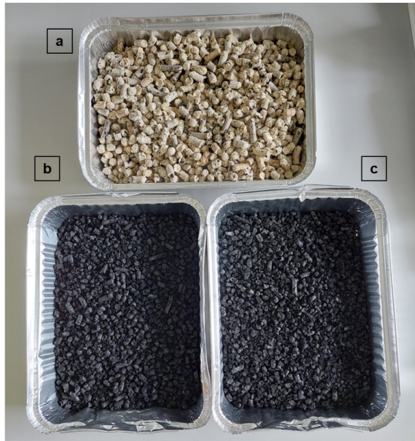
(a) 10% HDPE pellets, (b) 450 C, 20 min 10% HDPE biochar (c) 600 C, 20 min 10% HDPE biochar
