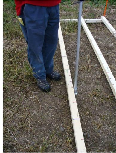
*Fig. 5: The surveyor's office surveying the soil surface with a measuring frame. Source: Agroscope ART*
