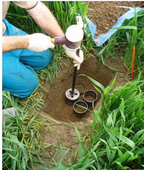
*Fig. 6: left: Panda penetrometer with measuring frame in the field. Right: Taking samples with core cutters to determine macroporosity. Source: Agroscope ART*
