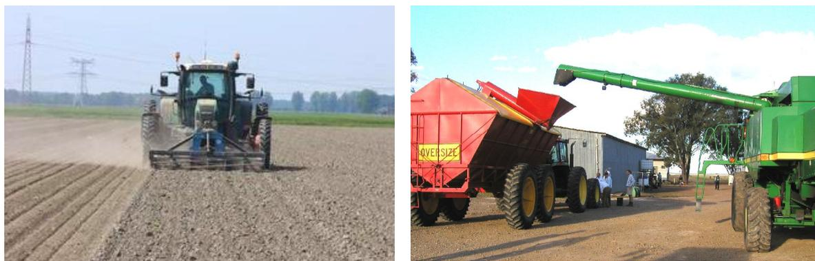
*Fig. 2, left: tractor with increased track width, right: grain hopper wagon and tractor with increased track width and combine harvester with lengthened grain auger. Source: Agroscope ART*
