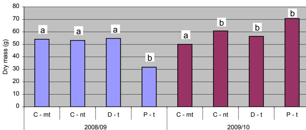
Fig. 10: Dry mass values after the intermediate harvests in April 2009 and 2010, statistical comparisons within each of the corresponding years. Legend: C-mt = controlled traffic - minimal traffic, C-nt = controlled traffic - no traffic, D-t = direct seed - trafficked, P-t = plough - trafficked. Source: Agroscope ART
