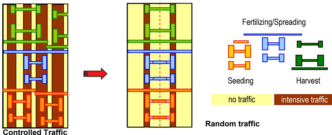
Fig. 1: Random traffic vs. controlled traffic. A large proportion of the surface is not trafficked, but
