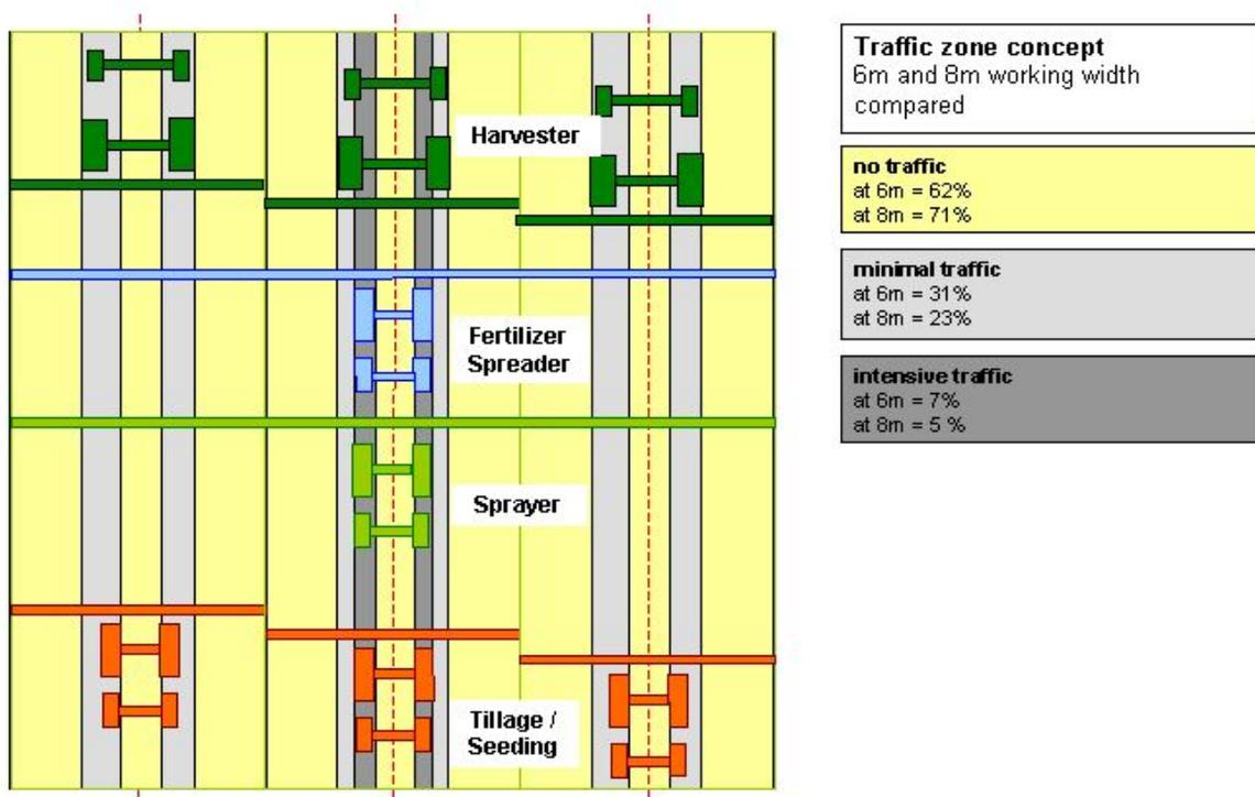
Fig. 4: Traffic zone concept: by including the areas of minimal traffic, 93-95% of the land is used for crop cultivation. Source: Agroscope ART
