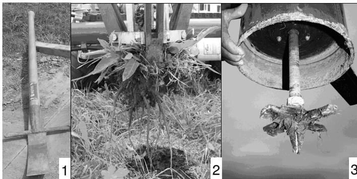
Fig. 1: Dock digger; Fig. 2: Mechanical weed grab; Fig. 3: Rotary-tiller element
