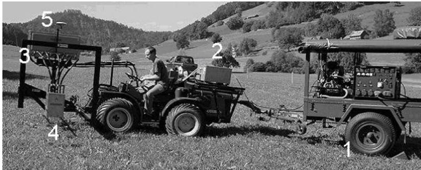
Fig. 4: Prototype I with 4.8 kW heat output
