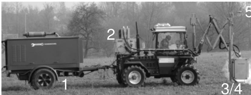
Fig. 5: Prototype II with 18 kW heat output
