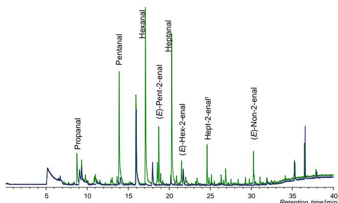
**Fig. 3:** Overlay of HS-SPME-GC-MS-chromatograms (total ion current TIC) of cream powder samples.
