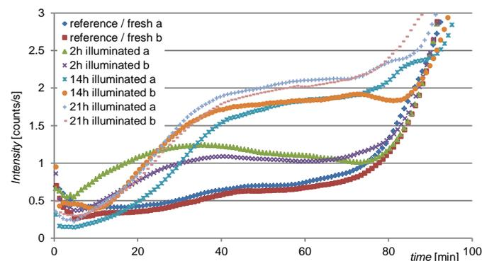
**Fig. 1:** CL-Measurements of roller-dried whole milk powder (heating rate 0.5°C/min, N<sub>2</sub> gas flow)
