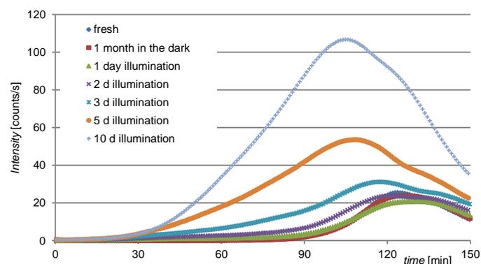
**Fig. 2:** CL-intensity of spray-dried cream powder show clear differences depending on illumination time (heating rate 0.5°C/min, N<sub>2</sub> gas flow)
