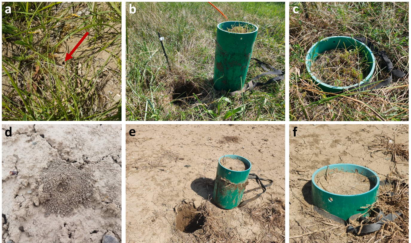
Fig. 2. Examples of two soil columns (b-c: column #1; e-f: column #7) used for repeated X-ray imaging. PVC tubes of 20 cm diameter and between 20 and 40 cm height were inserted using a tractor front loader at locations where at least one ground-nesting bee nest was found. (a, d) show examples of ground-nesting bee nests with visible nest entrances, indicated by the arrow in (a) and a typical tumulus (i.e., mound of excavated soil material) visible in (d) before the soil column was inserted. The black straps seen in the photos were used to pull out the soil columns for repeated scanning.
