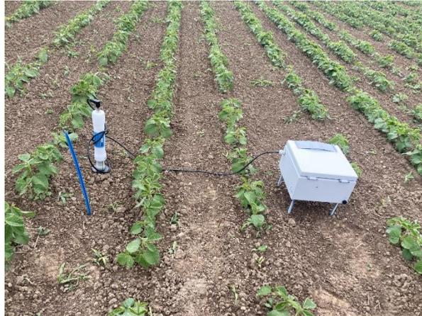
Figure 8: PR2 Profile probe with data logger (box on the right) on plot 8, 01/06/23.
