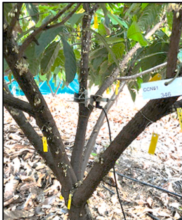
Fig. 2. Cocoa tree equipped with a dendrometer sensor and labels dividing the branches for weekly fruit counting.
