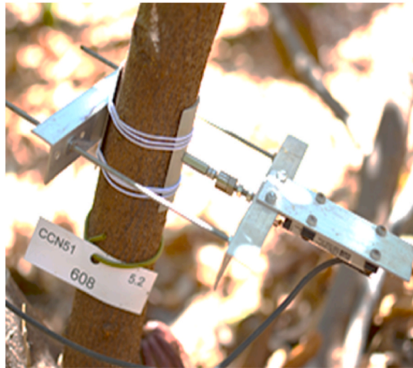
Fig. 4. Dendrometer installed on a cocoa tree in Juazeiro, Brazil.
