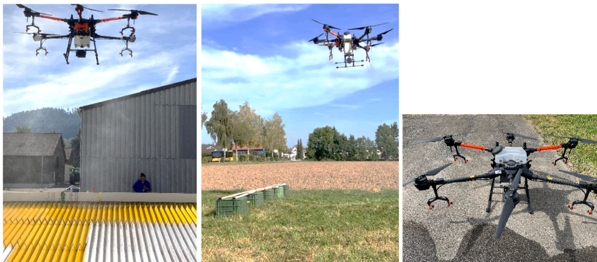
Fig. 1. UASS hovering over the patternator (left) and UASS flying over the slats fixing the strips of water sensitive and filter paper (middle), UASS DJI T16 with 2 nozzles per propeller on external motors (right).
