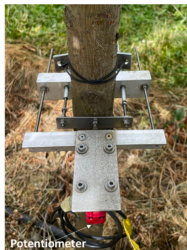
Fig. 2. Dendrometer constructed by Agroscope on the stem of an apple tree.
