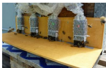
Fig. 2: Entrance board equipped with RFID-readers
