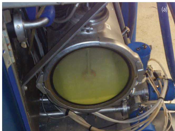
Figure 1a, 1b: Visible residues of milk in the end units of two AMS systems that are not adjusted well enough for milk sampling.
