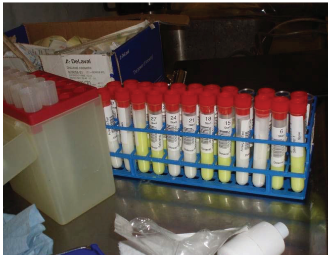
Figure 3: Test tubes with «Yellow», «White» and carry-over milk used in tracer method carry-over test.
