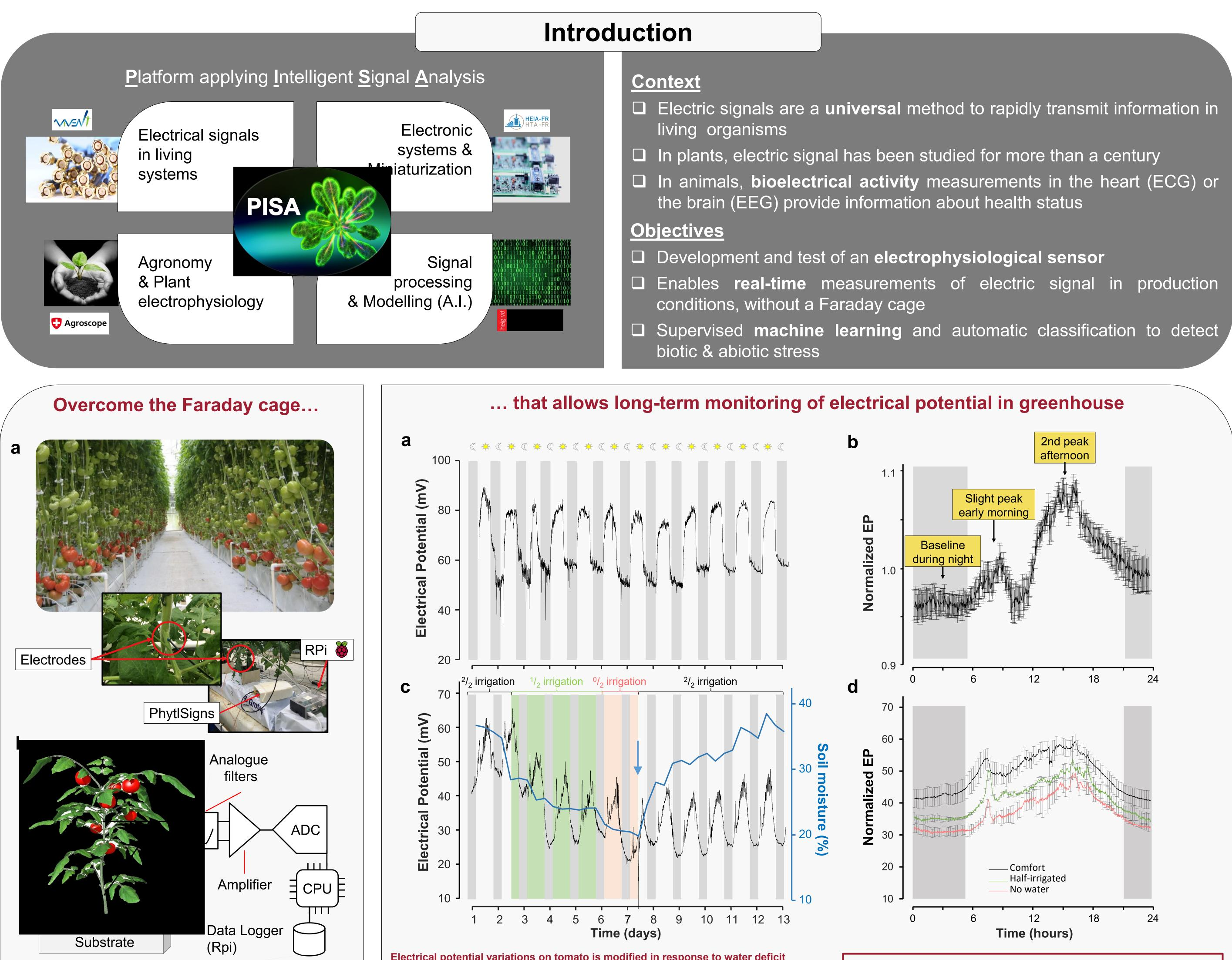
Enabling electrophysiological recordings outside a Faraday cage a, Experiments are performed on hydroponic tomato grown in greenhouse. The PhytlSigns device allows monitoring electric signal in 'real' environment without Faraday cage and electrode is inserted in the tomato petiole at the top of the plant (bottom). b, Schematic representation of the PhytlSigns composed of an amplifiervoltmeter and digitized data are collected into a Raspberry Pi.
