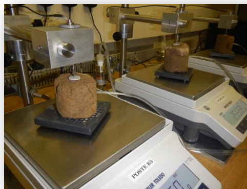
Figure 13: Soil shrinkage measurement: unconfined soil samples are drying on a scale, which is continuously measuring sample weight; sample height is continuously determined by a transducer; a micro-tensiometer is measuring continuously matric potential.
