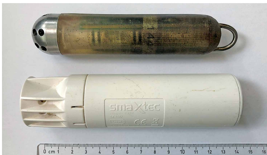
eCow bolus (top) and Smaxtec bolus (bottom) record continuously the pH in the reticulo-rumen of cows.
