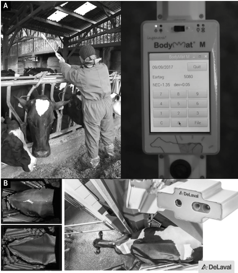
Figure 19.11. Two examples of BCS analysis devices available to commercial farms: (A) BodyMat from Ingenera; and (B) BCS by DeLaval.
