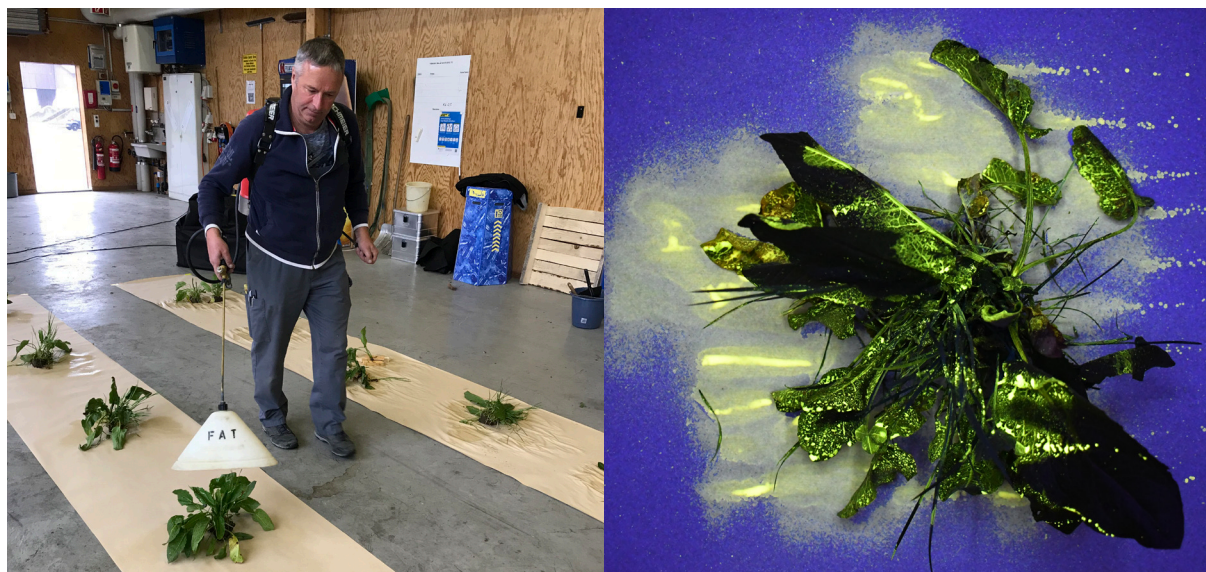
Figure 2: Spraying accuracy: dock plants were placed on brown paper lanes and treated with a spray liquid containing a fluorescent tracer (left); the sprayed areas were highlighted using UV light; the sprayed area around the plants (outlined around the plant), sprayed leaf area of the dock plants and unsprayed leaf area were determined (right) (© Agroscope)
