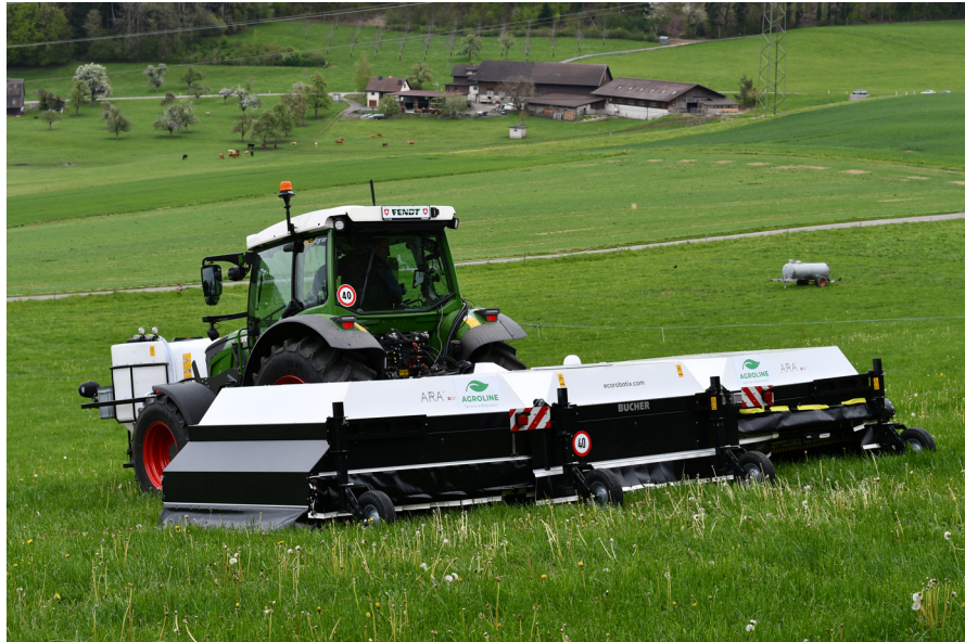
Figure 1: Spot sprayer Ecorobotix ARA treating broad-leaved dock plants in meadows (© Agroscope)
