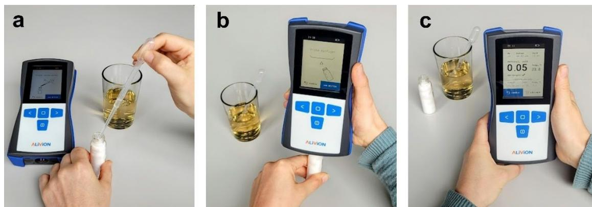
381 **Fig. 2** Measurement process with the *Alivion Spark M-20*. (a) Pipetting 2 mL of sample
