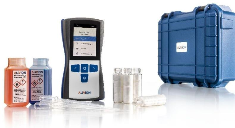
377 **Fig. 1** The *Spark M-20* with calibration standards, sampling vials, pipettes and carry case.
