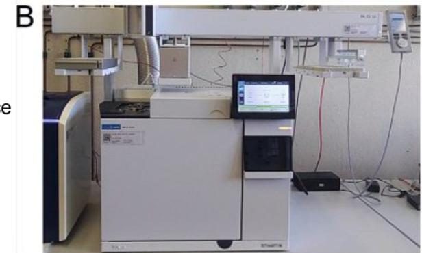
Agroscope's experimental cheese factory (A), Agilent 8890 gas chromatograph coupled with a flame ionization detector and a PAL3 autosampler in headspace mode (B).
