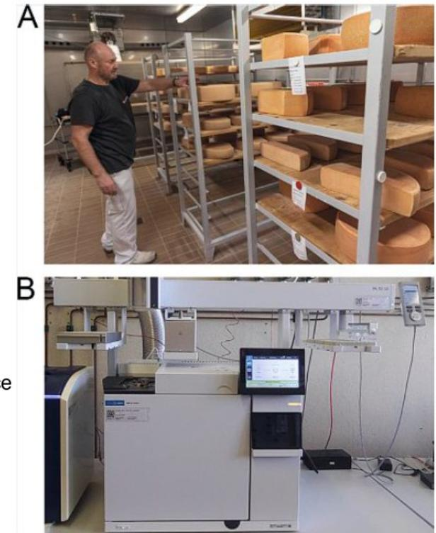
Agroscope's experimental cheese factory (A), Agilent 8890 gas chromatograph coupled with a flame ionization detector and a PAL3 autosampler in headspace mode (B).
