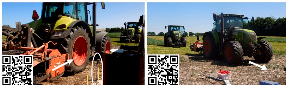
Fig. 1. Set-up in photo and video (QR-codes) of the main and facilitating tractors in the Passive (left) and Active (right) configuration. The white arrows indicate the driving direction. The white oval (left) highlights the laser-sensor (Section 2.2). Photos by Loraine ten Damme.
