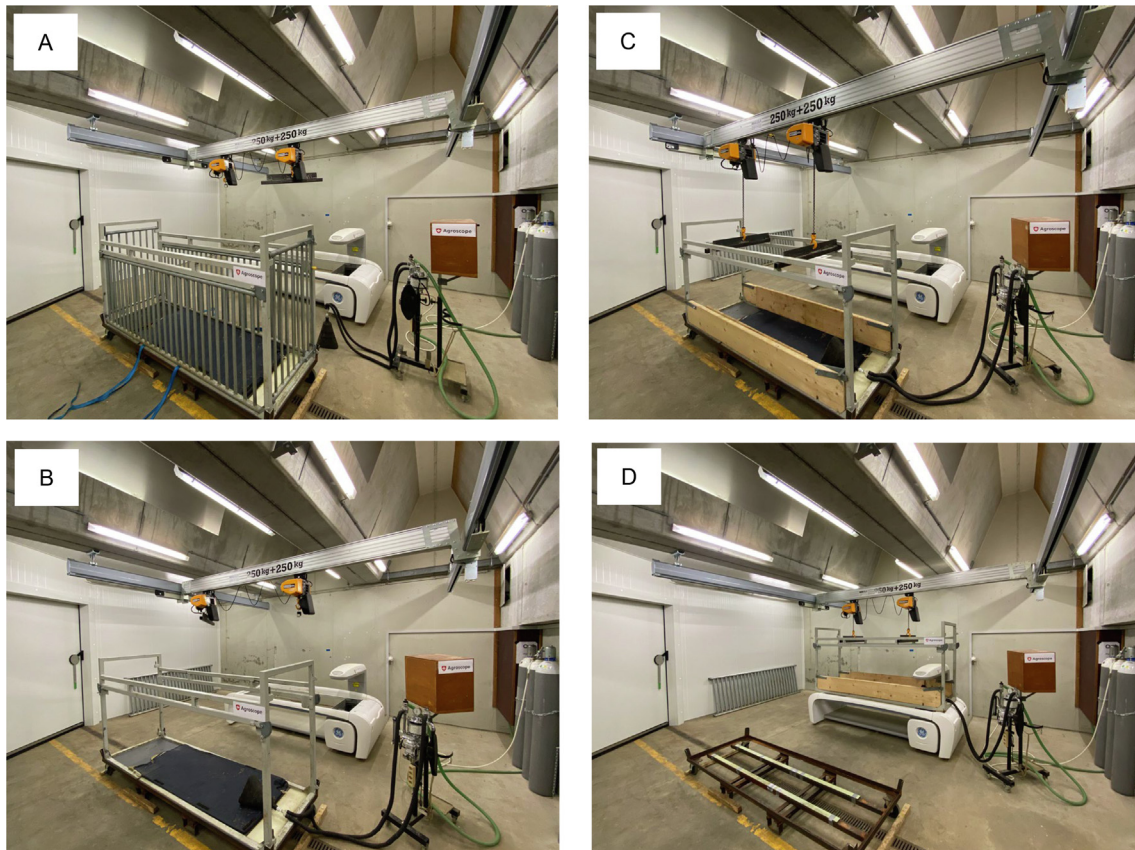
Fig. 1. Experimental set-up including restraint cage, anaesthesia and DXA device; A: cage setting for restraining the sow during until onset of anaesthesia; B: Cage setting for acquisition of an anaesthetised sow in ventral position; C: Cage setting for acquisition of an anaesthetised sow in lateral position; D: Cage positioned above the DXA device for acquisition procedure.
