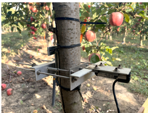
Fig. 2. Dendrometer sensor mounted on the apple tree in Grens, Switzerland.
