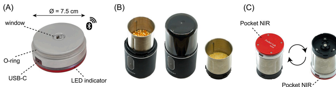
Fig. 1. The Pocket NIR with accessories. (A) Pocket NIR with glass window for scanning of the sample, O-ring for connection to the grinder container or sample cup, USB-C connector for charging, and LED indicator for on/off and battery status. Bluetooth logo indicates communication to the mobile app via Bluetooth LE. (B) Battery-driven grinder for sample preparation. (C) Pocket NIR connected to the grinder container. On the left, the situation with the Pocket NIR on top and the sample in the grinder container, i.e., the situation when displacing the sample by shaking. On the right, the situation with the Pocket NIR on the bottom and the sample on the Pocket NIR scanning window, i.e., the situation during a measurement. See the description of the measurement procedure in the main text.
