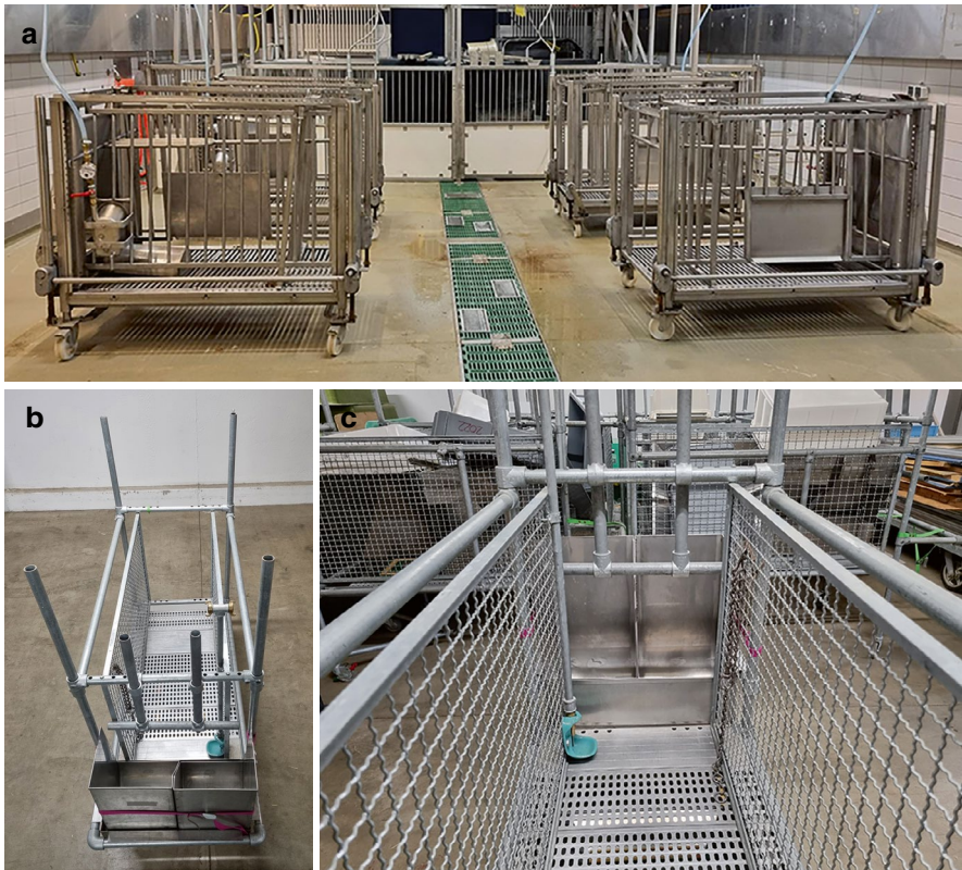
Fig. 5.1 Adjustable metabolic cages used at (a) FBN (Credit: Mariagrazia Cavalleri, FBN) and (b) Agroscope, with an example of (c) a feeding and water system (Credit: Marion Girard, Agroscope)
