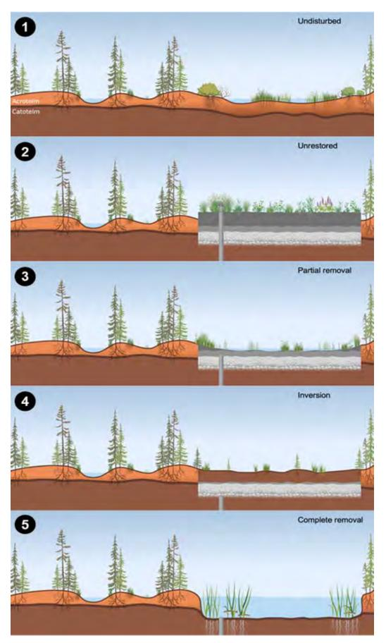
Figure 7.9. Schematic cross section of 1) a pristine peatland before disturbance, in comparison to the 2) unrestored peatland disturbed by infrastructures, and peatlands restored via 3) the partial removal of the mineral fill, via 4) the inversion of the mineral fill and the underlying peat, and via 5) the complete removal of the mineral fill, where a shallow open water area formed instead. Source: Lemmer 2022.
