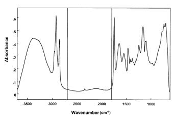
**Fig. 2** Typical mIR/ATR attenuated total reflection absorption spectrum using a Bio-Rad FTS-7 instrument; range of interest 3700–2700 and 1800–620 cm<sup>-1</sup>. Area between the *vertical lines* was omitted due to the low signal-noise ratio
