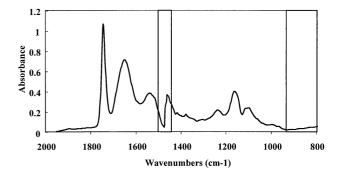
**Fig. 3** Typical mIR/Tr transmission absorption spectrum using a Nicolet Magna 750 instrument; range of interest 900 - 1450 and 1500-1800 cm<sup>-1</sup>. Area between the *vertical lines* was omitted due to the low signal-noise ratio
