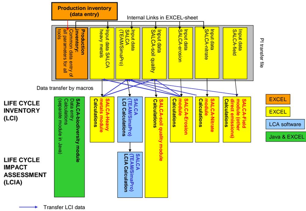
**Figure 1:** Modular architecture of the SALCAcrop calculation tool.
