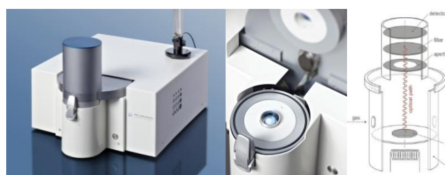
Fig. 2 Basic instrument configuration with the furnace cell and schematic view of the setup (ACL Instruments, CH-3210 Kerzers)
