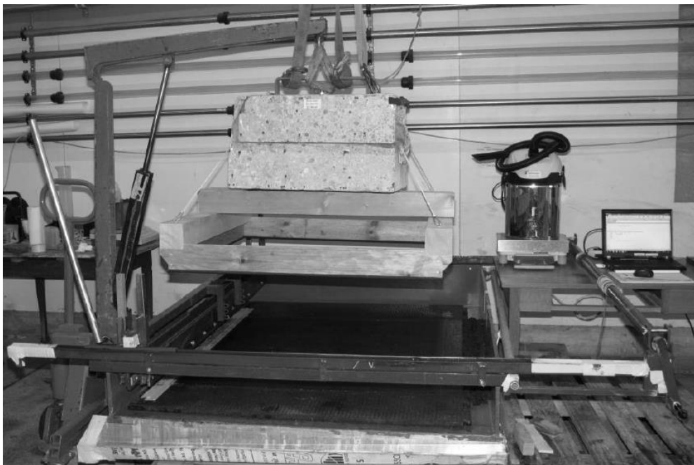
Figure 2: Pilot-plant experimental installation: Dung removal with the option of changing scraping tool and floor surface, with equipment for measuring residual soiling (frame, water vacuum cleaner, scales).
