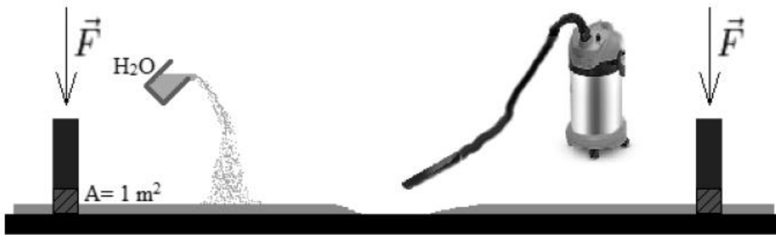
Figure 1: Scheme of the measuring method: Defined area with waterproofed frame; addition of water for dilution; vacuuming of residual soiling with water vacuum cleaner.
