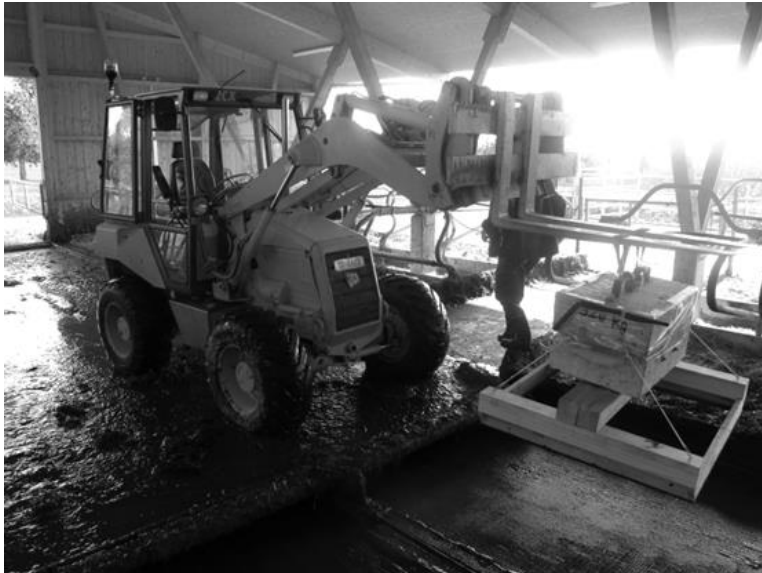
Figure 4: Handling of frame with weights between two residual-soiling collection processes on a feeding aisle in the commercial dairy housing
