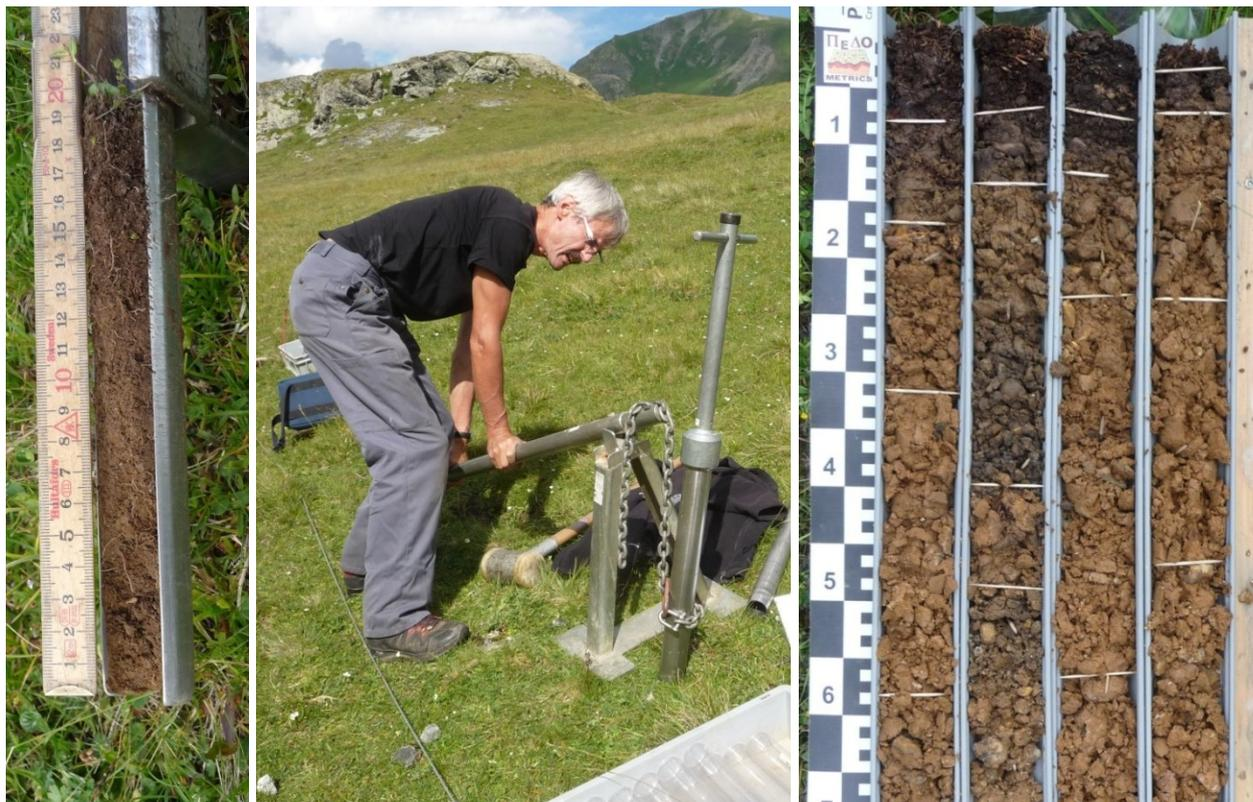
Figure 2: Left: subsample 0–20 cm used for composite sample. Middle: extraction of a soil core by a core sampler at a grassland site. Right: soil cores collected in a coniferous forest (site 83). The displayed soil layers correspond to organic layer (top), A horizon, AB horizon, B horizon, and BC horizon (bottom).
