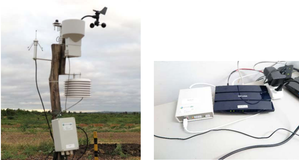
Figure 65: Left: Weather station: Wind direction and speed, pluviometry, pyranometer, temperature and air humidity and RF-Antenna. Right: Modem and Internet connection.
