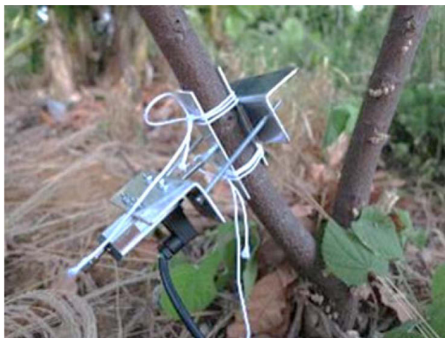
Figure 22: Dendrometer measuring the variation of stem diameter of a main tree branch.
