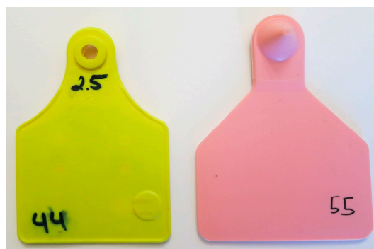
Figure 1. (left): ultra-high frequency (UHF) ear tag Type A, (right): UHF ear tag Type B.
