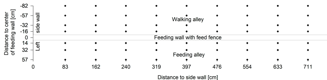
Figure 3. Coordinate grid for reading range measurements in front and behind the feed fence. Measurements were conducted at heights of 30, 55, 80 and 105 cm above the floor. Each x-coordinate represents the centre of a feeding place along the feed fence.
