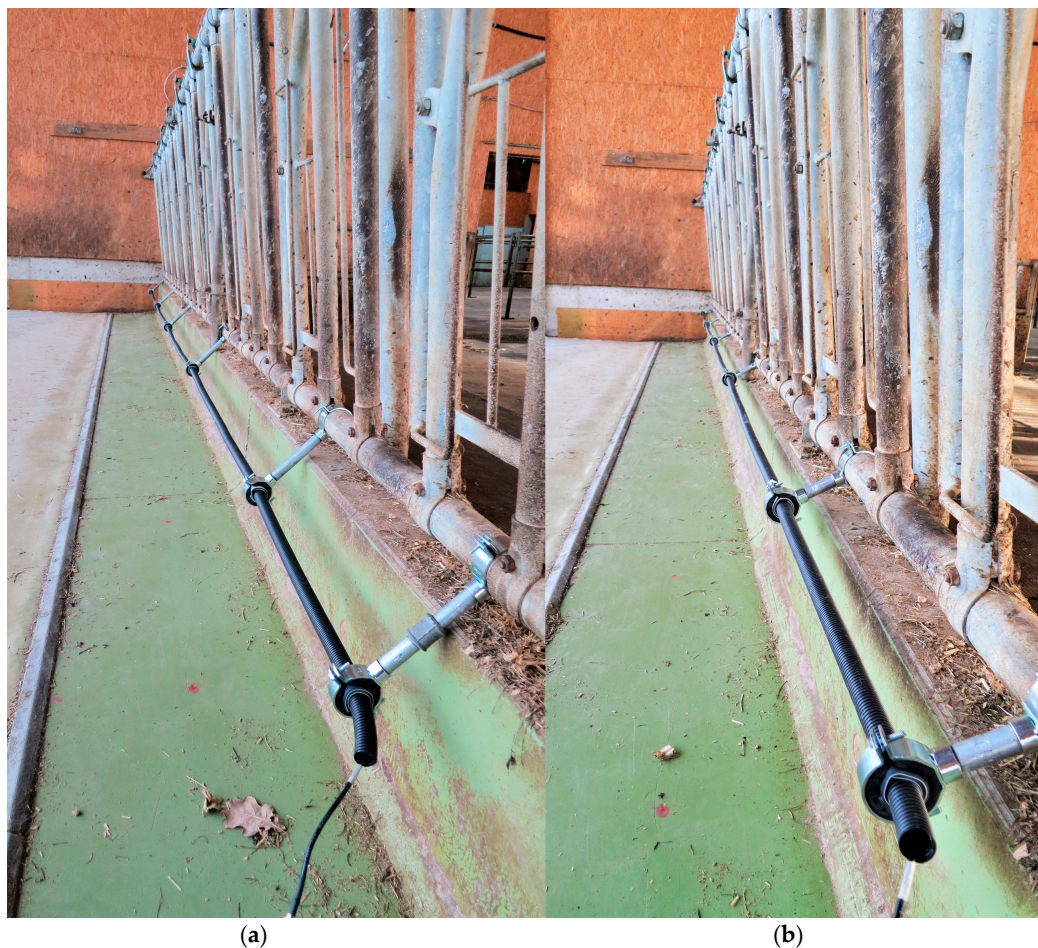
Figure 2. Setup of the antenna at the feed fence. (a) Antenna Position 1; (b) Antenna Position 2.
