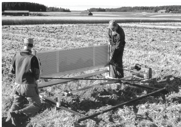
Figure 4. A soil roughness meter is used to measure changes in the surface of soil. Photo: Risto Seppälä, Natural Resources Institute Finland (Luke).
