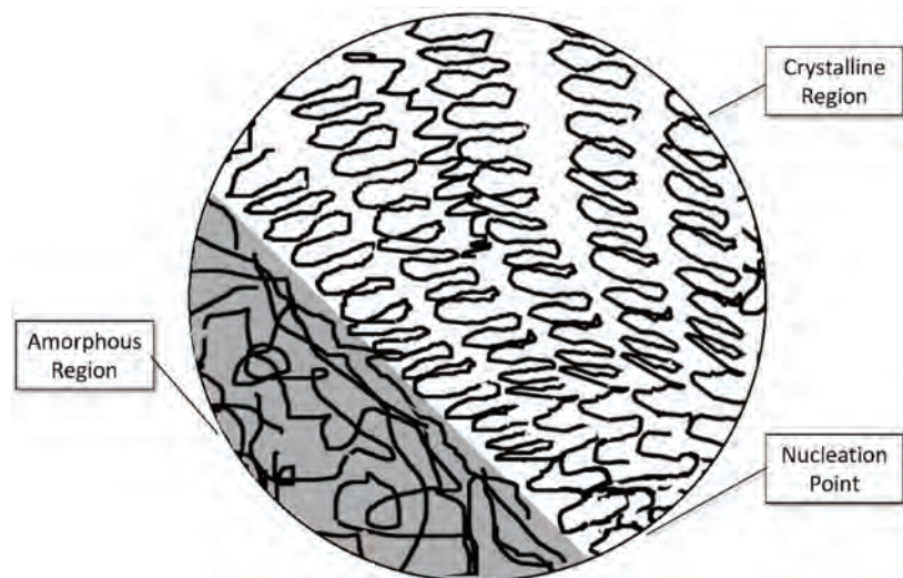
Figure 2. Illustration of highly ordered polymer chains in crystalline regions and disordered chains in amorphous regions.
