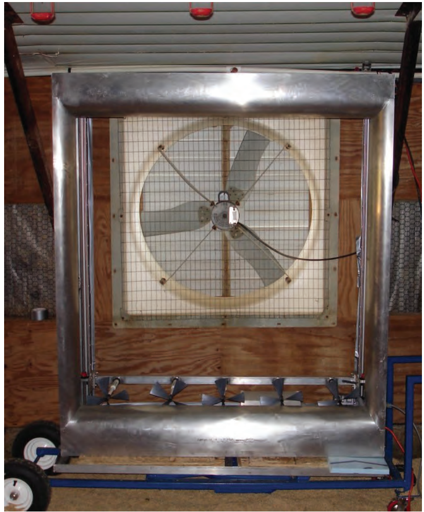
Figure 10. Fan assessment numeration system (FANS) developed by Gates et al. (2005) to describe the performance curve of a ventilation fan in an animal house. The unit can be used on either the inlet or exhaust side of the ventilation fan.
