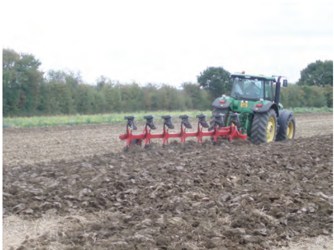
Figure 13. Tractor-mounted moldboard plow working in the field.
