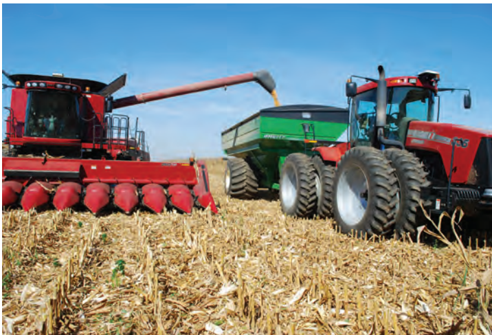
Figure 11. Typical grain cart receiving clean grain from a combine.
