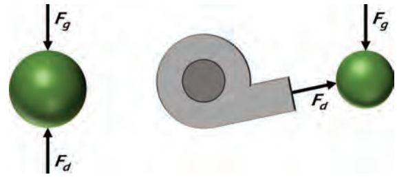
Figure 4. Forces affecting particle motion when it is free falling (left) and when subjected to a directed air flow (right).
