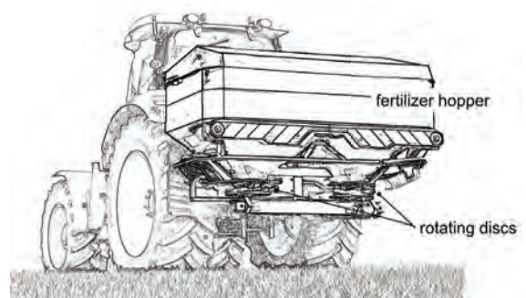
Figure 19. Centrifugal fertilizer spreader mounted on the three-point hitch of a tractor.
