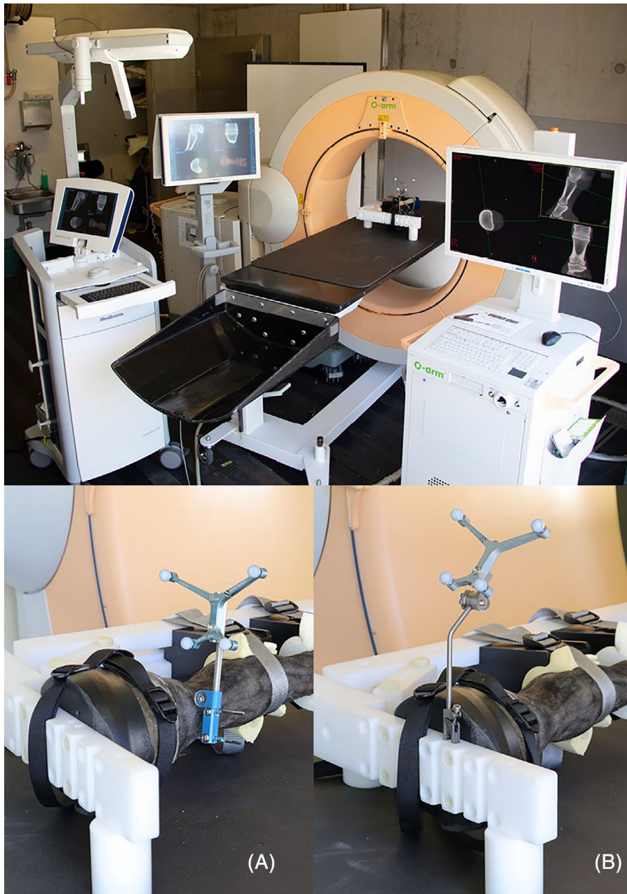
FIGURE 2 The computed tomography-based surgical navigation system immediately after image acquisition. The cadaveric limb is secured in the purpose-built frame and placed on a carbon table. A, The tracker is anchored to the dorsal aspect of the proximal phalanx using two 3.2-mm pins as distal as possible (control group). B, The tracker is anchored directly to the frame (study group)
