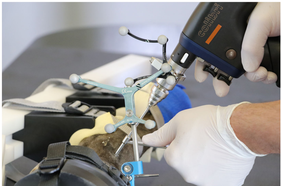
FIGURE 4 Spatial interference during a drilling procedure. The patient tracker (anchored to the proximal phalanx, control group) and the instrument tracker mounted on the drill are superimposed, impeding proper detection of the trackers by the localizer camera
