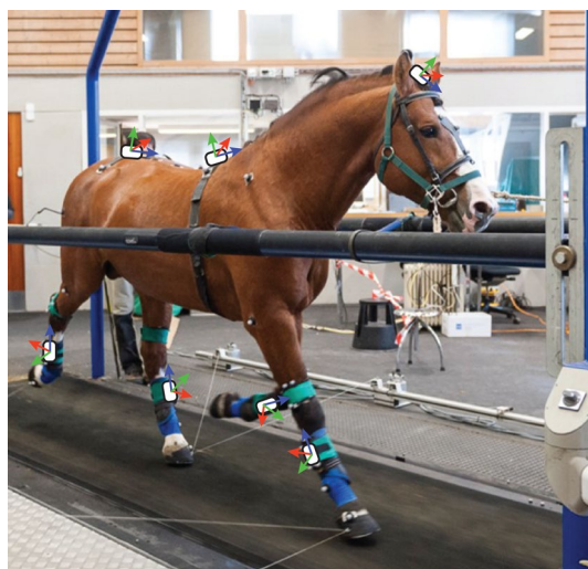
Figure 8. Horse on the TiF, equipped with reflective markers of the OMC system and the IMU nodes (white rectangles). Orientations of the nodes are shown with blue (x-axis), red (y-axis) and green (z-axis) arrows. Copyright: Erns A. Kehrlı–Vetcom UZH.
