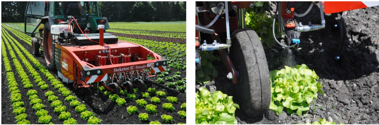
Fig. 1. Prototype based on a camera-controlled hoeing machine (left) with added spot-spraying technology for targeted pesticide application (right). Source: Agroscope, R. Total.
