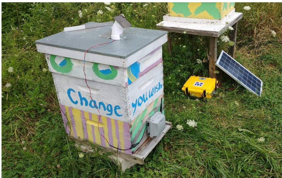
Figure 12. Beehive activity monitor (including a Doppler radar) located above the entrance of a hive, with solar panels as energy sources (from Cunha et al., 2020 with permission).
