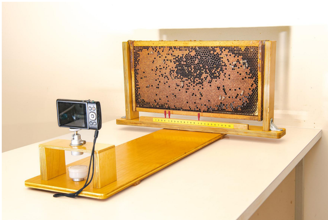
Figure 6. Mount where a comb is placed in a holder and the distance between the comb and camera is fixed to photograph its sides.
