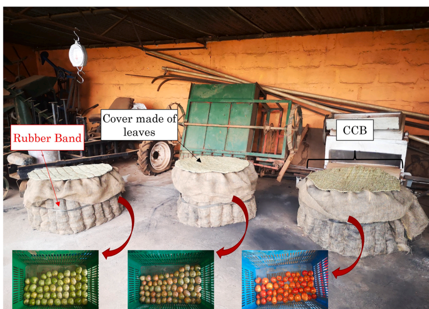
Fig. 1. Three filled charcoal cooling blankets (CCB) wrapped around three plastic crates of tomatoes at different ripening stages (green, breaker, red) and kept inside the shelter showing the rubber strap tied around the CCB and the leaf cover on top of the blankets.
