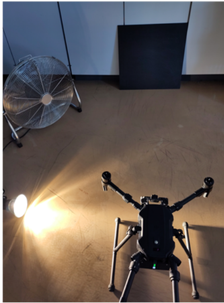
FIGURE S2.4: Setup of fan experiment. The drone was pointing at a PVC sheet. From an oblique frontal angle, the fan was blowing in the direction of the sensor. From the side, a lamp was heating the sensor without directly pointing into the FOV of the camera.
