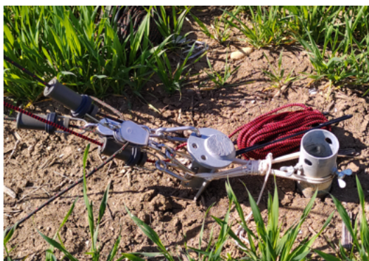
FIGURE S3.2: A ground screw was used to reinforce anchor pins. The pins are prone to loosening with the mast continuously shaking slightly in the wind.
