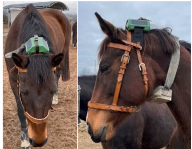
Fig. 1. Research Device (RD) mounted on halter for horses. The RD is placed on the horses' neck. The grey box on the collar contains an independent GPS unit for comparative data quality analysis.
