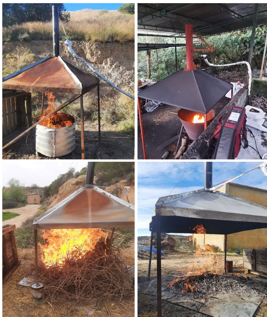
FIGURE 1 | Kon-Tiki kilns with 150L (top left) and 1000L (top-right) with hood and chimney to collect and channel flue gas emissions to the analyzer probe. Open burning of orchard pruning (bottom), directly after ignition (left) and towards complete combustion (right). A sketch with dimensions of Kon-Tikis, fire place, and hood is shown in Figure S1.
