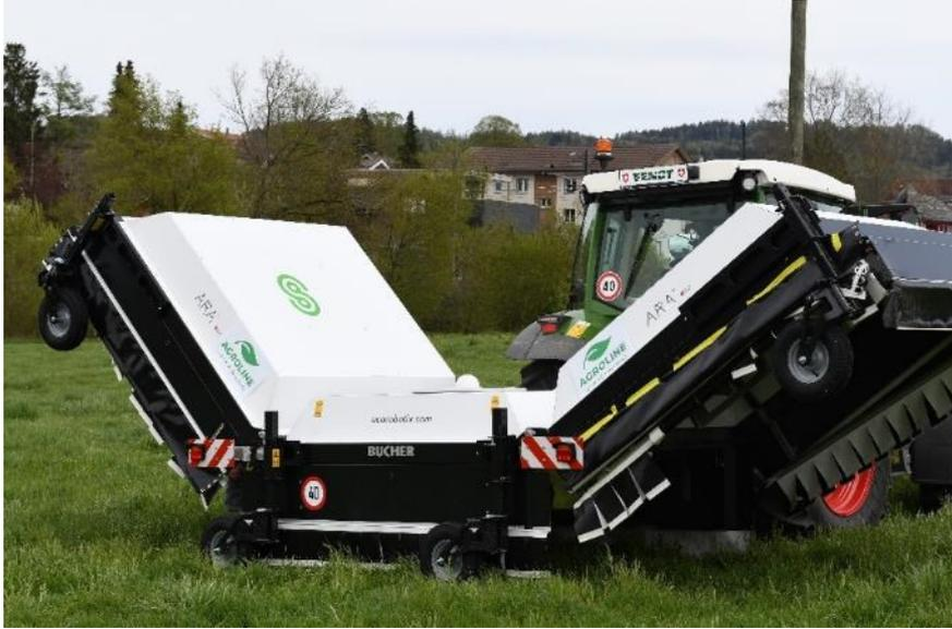
3 independent units equipped with cameras, 6 m working width
