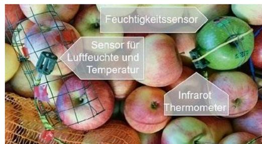
Abb. 2: Kondensationsmessung. (© Agroscope)
