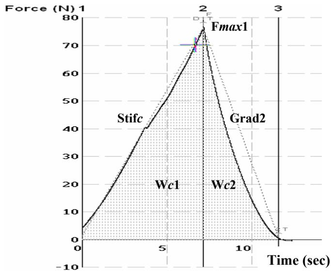
Fig. 2. Force-time curve from compression measurement.
