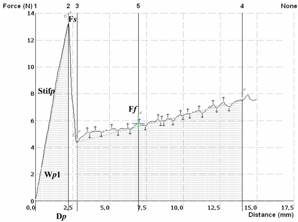
Fig. 1. Force-displacement curve from penetrometric measurement.
