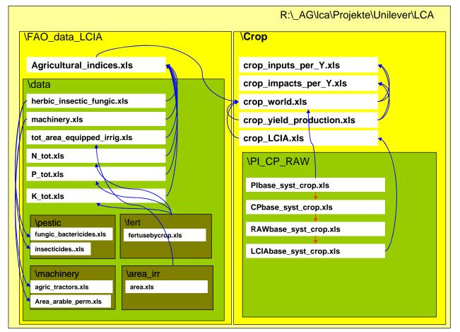
Fig. 4-1. File System for the modular inventory. The coloured rectangles are folders, the white ones are files, and the blue arrows are the symbolic links between the files, red arrows show the order of the calculations within the SALCAcrop tool. Crop corresponds to the studied crop and Y is either kg or ha.
