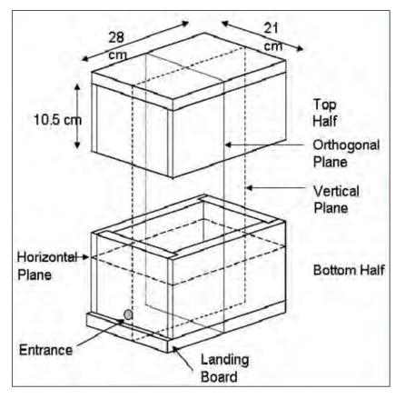
Figure 4: Diagram of the hive box designed by Dr Tim Heard for T. (reprinted with permission from the Australian Native Bee Research Centre) and showing planes of scanning.
