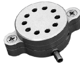
Figure 2: Impactor and conditions for sampling and gravimetric determination.
