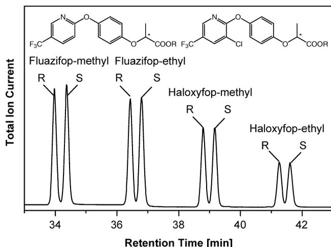
**Figure 1.** Reconstructed ion chromatogram of eight mass traces showing the elution of the enantiomers of haloxyfop-methyl (concentrations, 1.7 mg/g plant dry weight), haloxyfop-acid (analyzed as ethyl-ester, 1.0 mg/g), and the corresponding internal standards (fluazifop) in an ethylated extract from blackgrass, sampled 24 h after treatment with *rac*-haloxyfop-methyl. Nonenantioselective metabolism was observed for both methyl-ester and acid.
