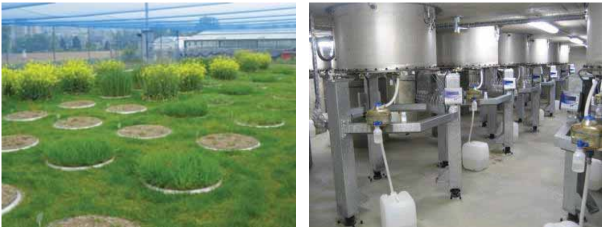
Fig. 1. Lysimeter facility: above-ground part with temporary grassland, sugar beets and oilseed rape in the year 2011, and basement with the weighing lysimeters.
