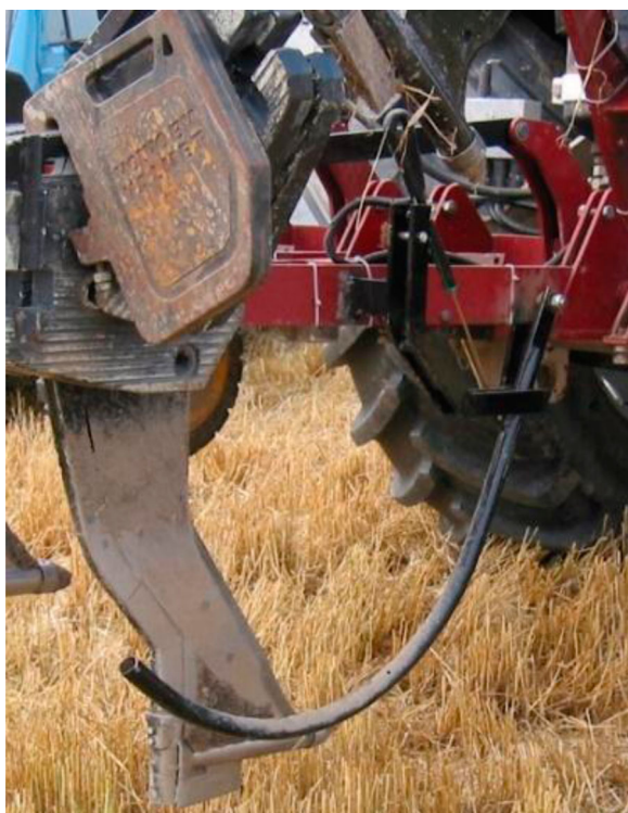
Figure 3. The depth measuring system. The curved metal pipe followed the soil surface and was attached to the metal frame. The angle was measured and from that the depth of the cones could be calculated.
