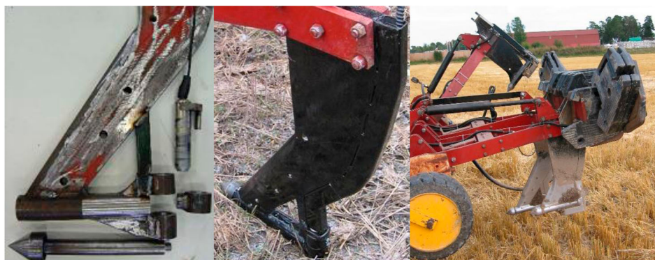
Figure 2. Detailed picture of a soil penetrating cone, mounted soil penetrating cone and all three soil penetrating cones.
