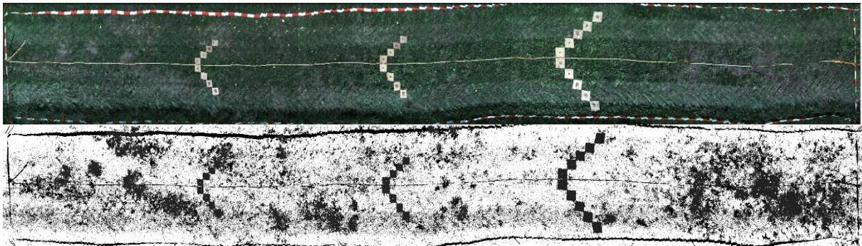
Figure 2: test field with wooden plates simulating gaps in meadow
