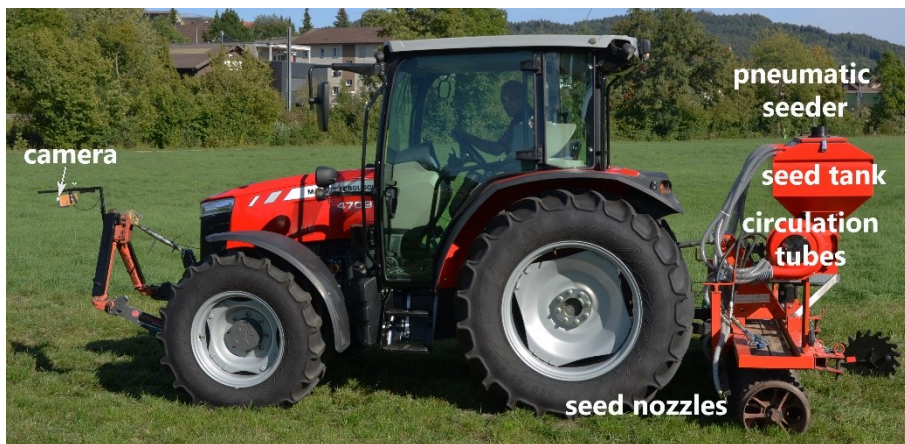
Abbildung 1: tractor with camera in front and seeder at the back
